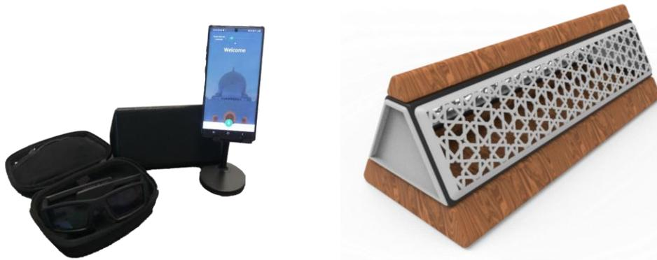
**Figure 2.** Components of IMAM - Mobile App, smart speaker, and intelligent eyeglass
