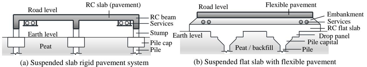
(a) Suspended slab rigid pavement system
