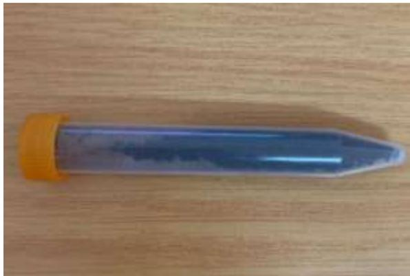
Figure 2: Produced nano zero valent iron stored in closed medium
