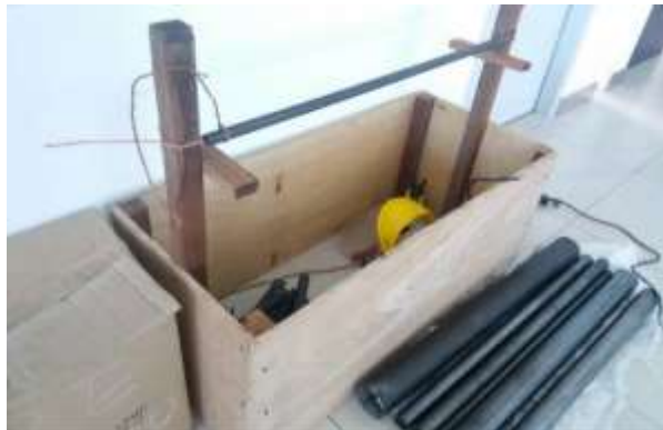
Figure 4: Wooden support showing six carbon steel pipes
