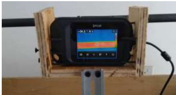
Figure 3: FLIR camera showing the temperature gradient on a pipe
