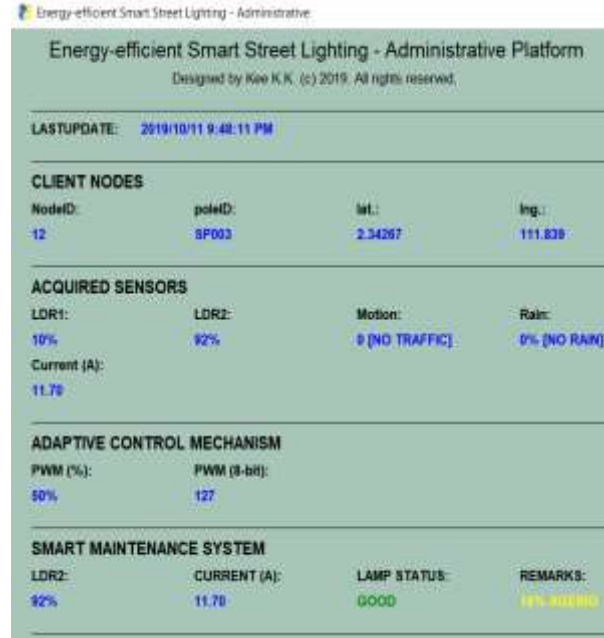
Figure 18: Visual Interface showing the mesh clients information
