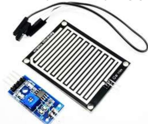
Figure 11: Rain/Water Sensor
