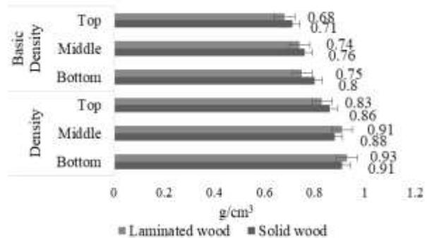
Figure 2: Density and basic density for solid wood and laminated wood due to the different portion
