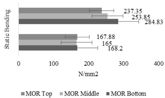
Figure 3: Modulus of rupture for static bending test on solid wood and laminated wood due to the different portion
