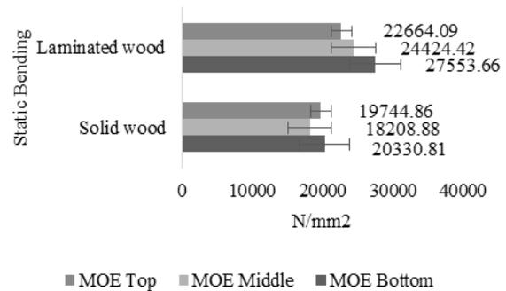
Figure 4: Modulus of elasticity for static bending of solid and laminated wood at a different portion
