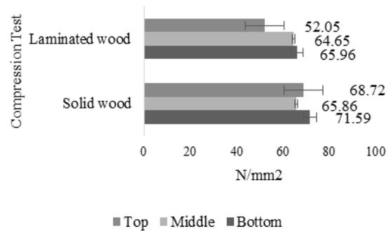
Figure 5: Compression test on solid wood and laminated wood due to the different portion.
