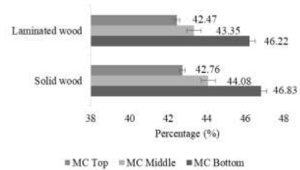
Figure 1: Moisture content for solid wood and laminated wood due to the different portion.
