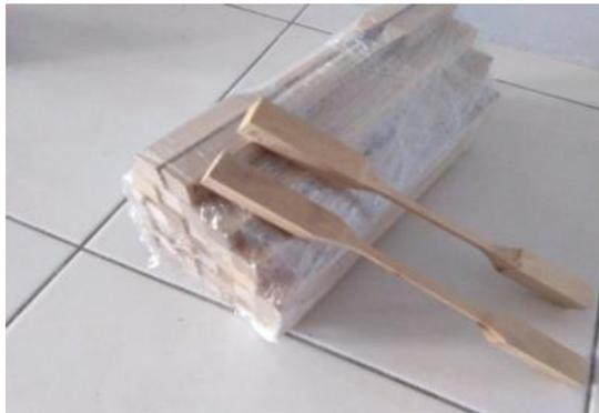
Figure 1: Dog bone shaped tensile test specimens
